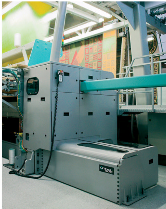
Stäubli Unival 500 electronic shedding mechanism
